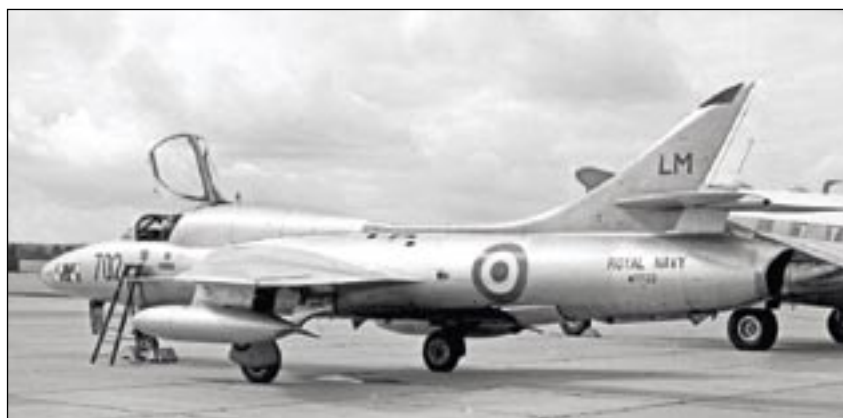
ABOVE Another of the aircraft John Middleton flew during his conversion to fast jets was the Hawker Hunter T.8. This Lossiemouth-based example, WT722, operated with 764 NAS, and is seen in the standard colour scheme of aluminium finish with dayglo orange-red trim.
